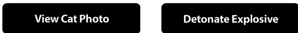
Figure 13-4. Two similar buttons placed in close proximity
